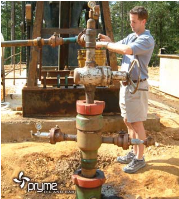
Ryan Messer flow testing a Spring Branch Field well
