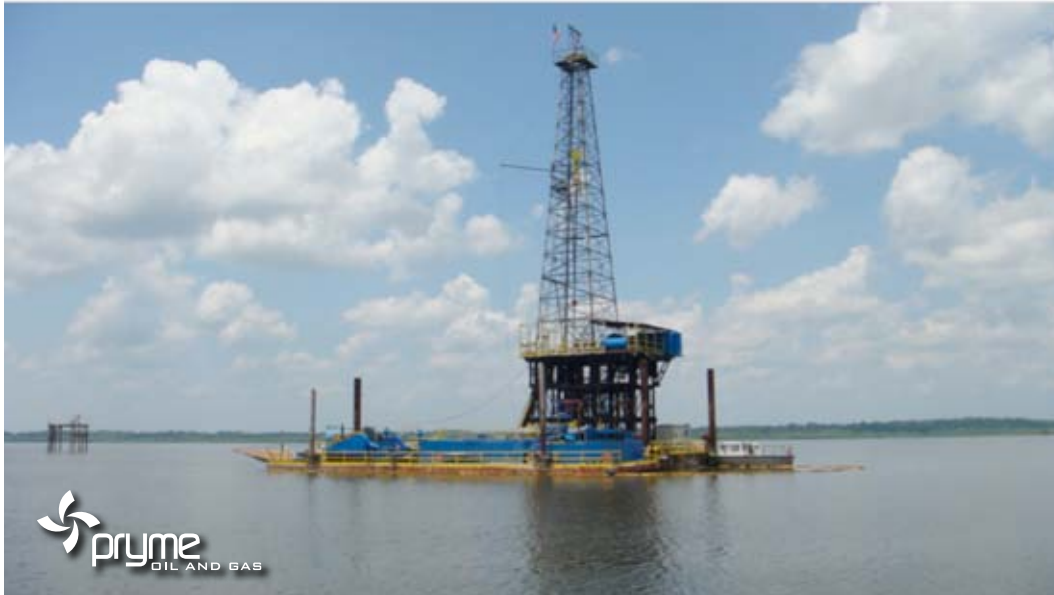
Drilling the SL 502 No.1 from the barge mounted rig in Catahoula Lake, Louisiana
