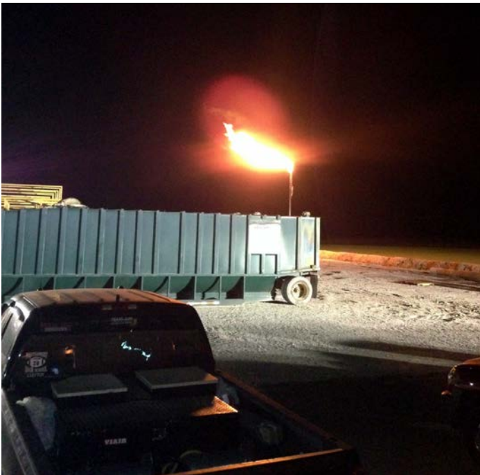
Flaring natural gas during flow back of RP21H
