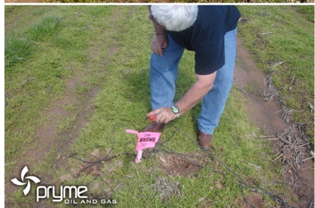
Woody Dunn (Weems Geophysical field superintendent) inspecting fuse wire connected to field charges and receiver lines within the 3-D shoot
